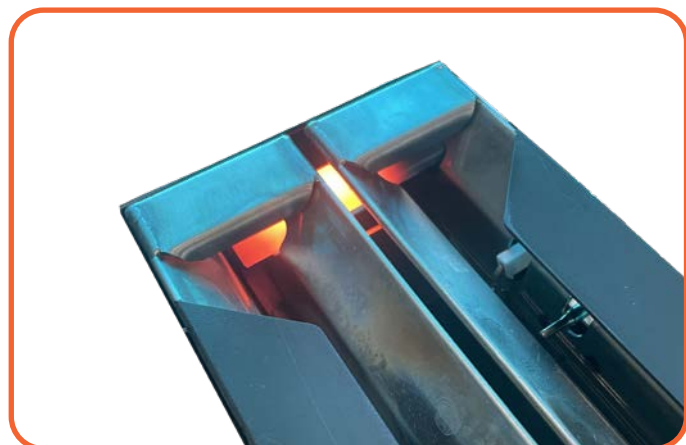
Figure. 4.5 PRIMING: Fuel is going to be ignited
